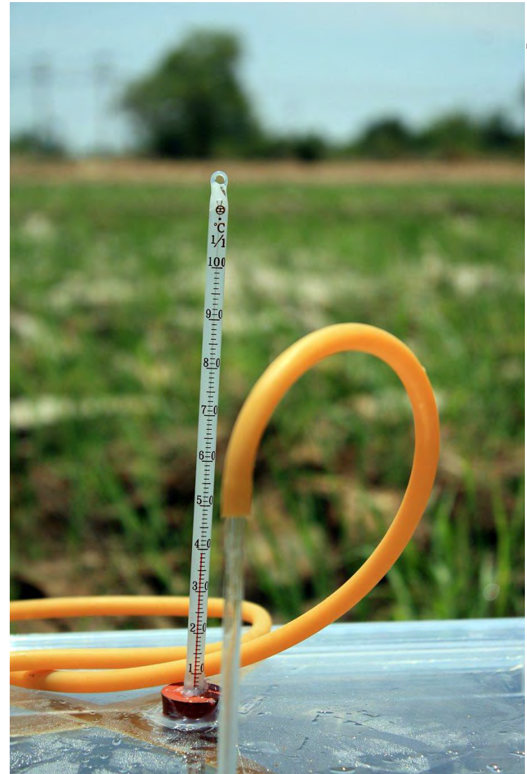
A thermometer and a sampling hole covered with a rubber septum.
